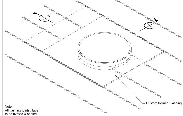
**ROUND ROOF WINDOW** STANDING SEAM ROOFING PROFILE PITCH 5° TO 60°
