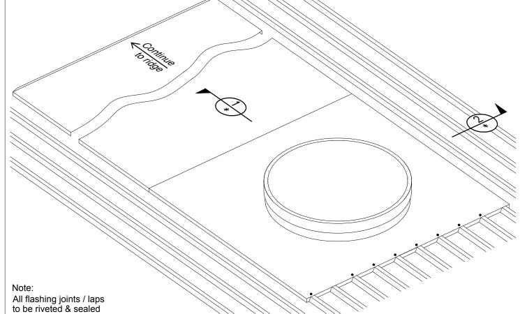
ROUND ROOF WINDOW TRAPEZOID ROOFING PROFILE (Back Tray) PITCH 5° TO 60°
