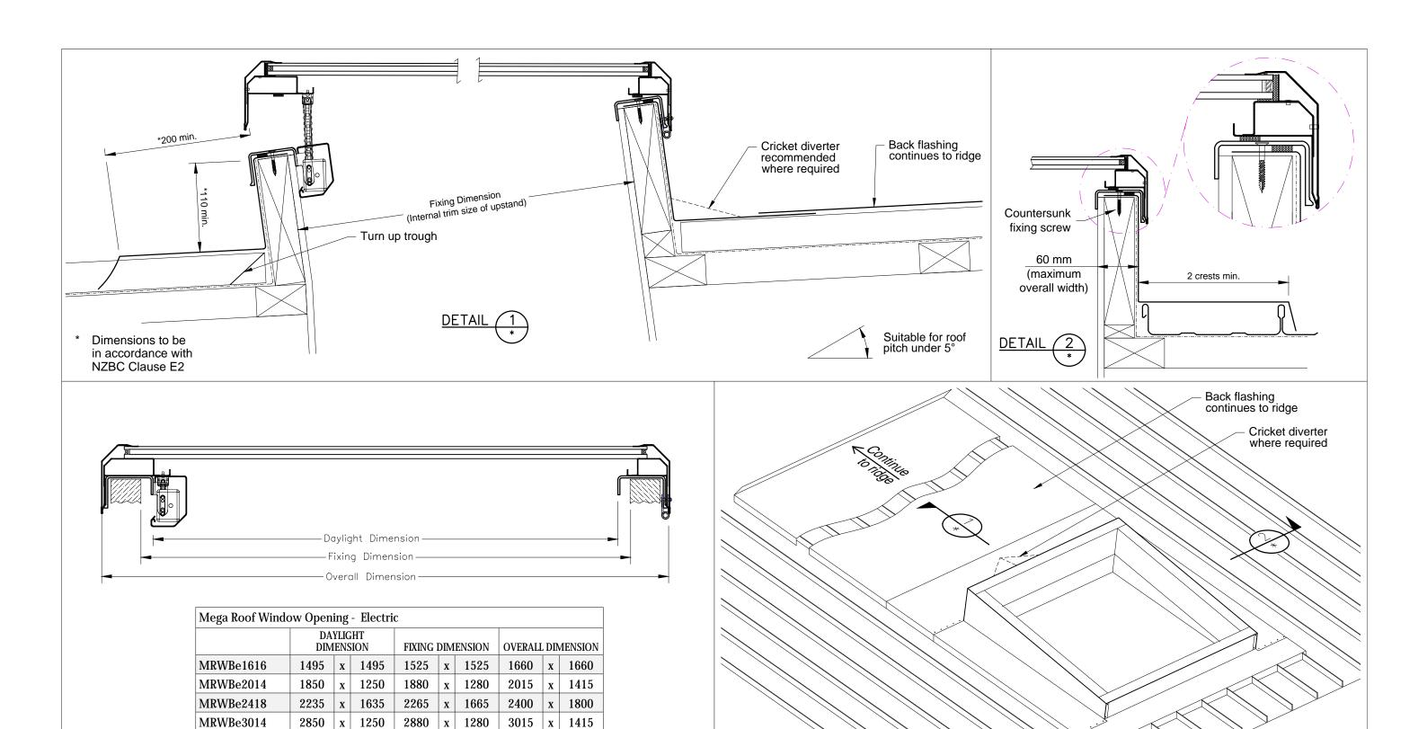
Not to scale, do not scale from drawing. All details are generic in nature and should be read in conjunction with the roofing manufacturers' standard penetration details.
